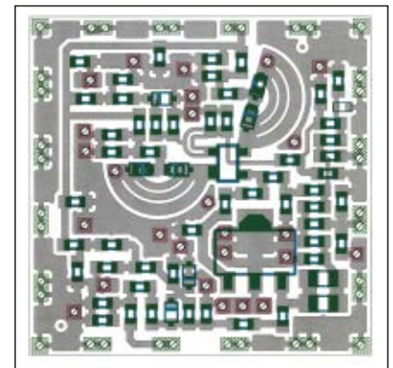
Fig. 3 Layout of the 2 to 6 GHz coupled resonator VCO (patent pending).
