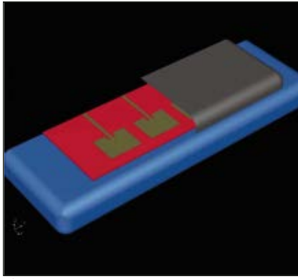
▲ Fig. 1 A four-element planar patch array as imported from Microwave Office into MicroStripes 7.5 where additional 3D geometry has been added.
